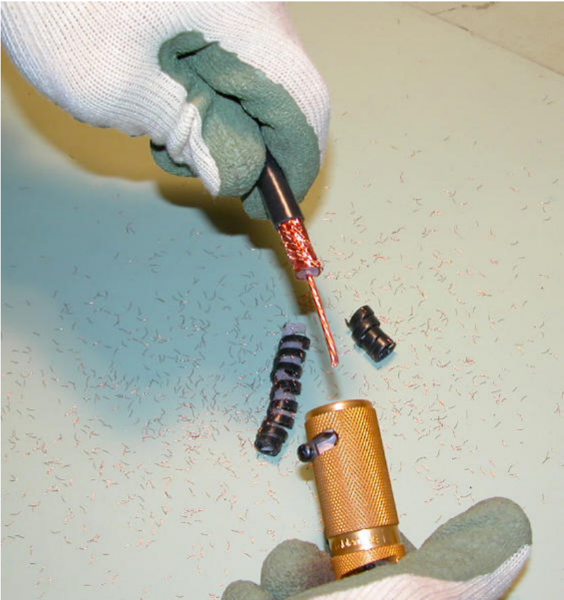
LOOKING AT COAX WITH OUTER JACKET REMOVED
